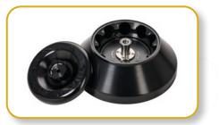
**Fixed-angle Rotor** Aluminum rotor for ten 50 ml conical tubes. It has available adapters for 15 ml conical and dome tubes.
